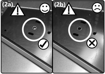
Ensure that the seat shell is firmly anchored to the seat plate and cannot be pushed forward.
