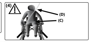
The seat belts must not be twisted during use, nor must they be guided over any structural components, which would keep them away from the body. They have to be tight and firm without impairing user comfort. The lap belt buckle must be positioned between the pelvic bones (if possible in the middle). The buckle tongues on the lap belt for fastening the shoulder belt should be located on the outside of the pelvis where possible.
