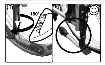
Only rotate the anti-tipper 180° from deactivated position to active position. Avoid full revolutions in one direction, since otherwise the tension spring inside the anti-tipper will be damaged, which may result in the anti-tipper losing its functionality.
