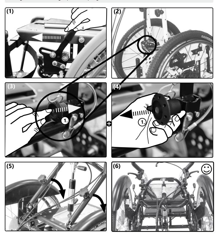
Folding open back with gas pressure spring: Proceed accordingly in reverse order:
