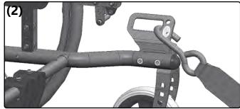
The seat shell-underframe must be fixed with a 4-point wheelchair restraint system anchored to the vehicle in accordance with ISO 10542. These may be carabiner hooks, S-shaped hooks or plug-in fasteners. The wheelchair restraint system must be securely fastened and used in accordance with the user manual of the manufacturer. (3A+B)
