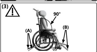
If the seat shell-underframe is equipped with a back angle-adjustment or tilt mechanism, the occupant must sit in an upright position at a 90° back angle during transport (3). Leg supports that can be swung up must be adjusted to the lowest position.
