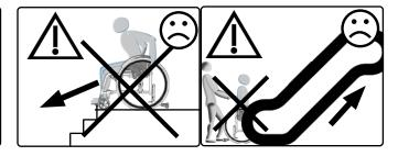
Only negotiate stairs with the help of experienced assistants. The anti-tipper must be deactivated when doing so. The seat-shell underframe must always be carried by the frame only, never by the seat shell, the extendable push handle(s), push bail, handle bar, leg supports and/or the footrest(s)!
