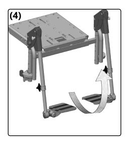
Leg rest can be detached, folded down and adjusted in width with continuous (5a) or divided footrest (5b)
