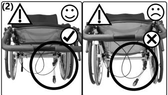
The anti-tipper must always be locked in its end position.
